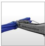
4. Place front of nosepiece flush to the head of the cable tie.
