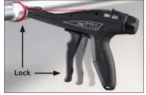
The locking mechanism detects when the desired tension is reached, locking the tie in place prior to cutting. No manual pressure is required to hold the cable tie in place.
